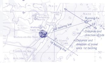
When only one object is visible, you can use a procedure called a 'running fix' or 'transferred position' line to work out your approximate position.
