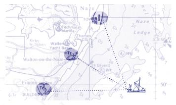
Take a bearing of three fixed objects and draw the appropriate bearing to seaward on the chart. Where the lines cross is your position.
